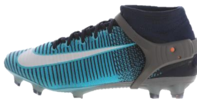
Figure 1. An image of the Playermaker device and how it is fitted to the lateral malleolus of the foot
